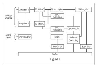
The block diagram of the board DA 1250 is shown in figure 1.
